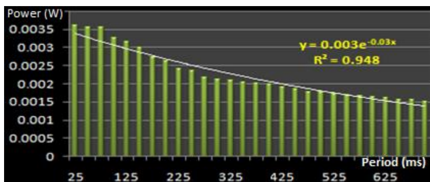
Figure 4. Power consumption versus transmission period.
